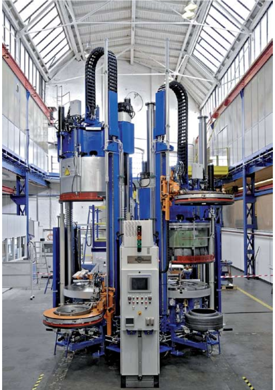
HF designed the first hydraulic curing press, the first column-type press, and the first platen type press and has now released a new truck tire press design with the Truck Tire Press Type 67-450 H
